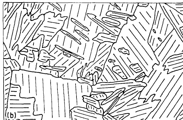
Figure 2 Illustration of artificial etching in order to reveal the \alpha colonies and their schematic orientation. (a) Original microstructure of a TA6Zr5D alloy. (b) Ink etching of (a).
